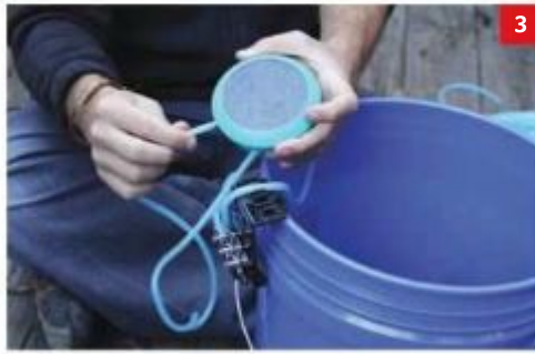
(3) Cut three more pieces, each long enough to reach from the rim of the bucket to its bottom, and attach those to a port of the gang valve on one end and a bubbler on the other.
